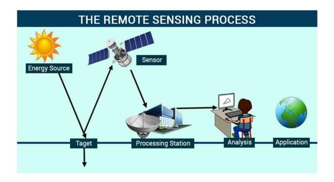
The remote sensing process involves an interaction between incident radiation from an energy source and the targets of interest.
